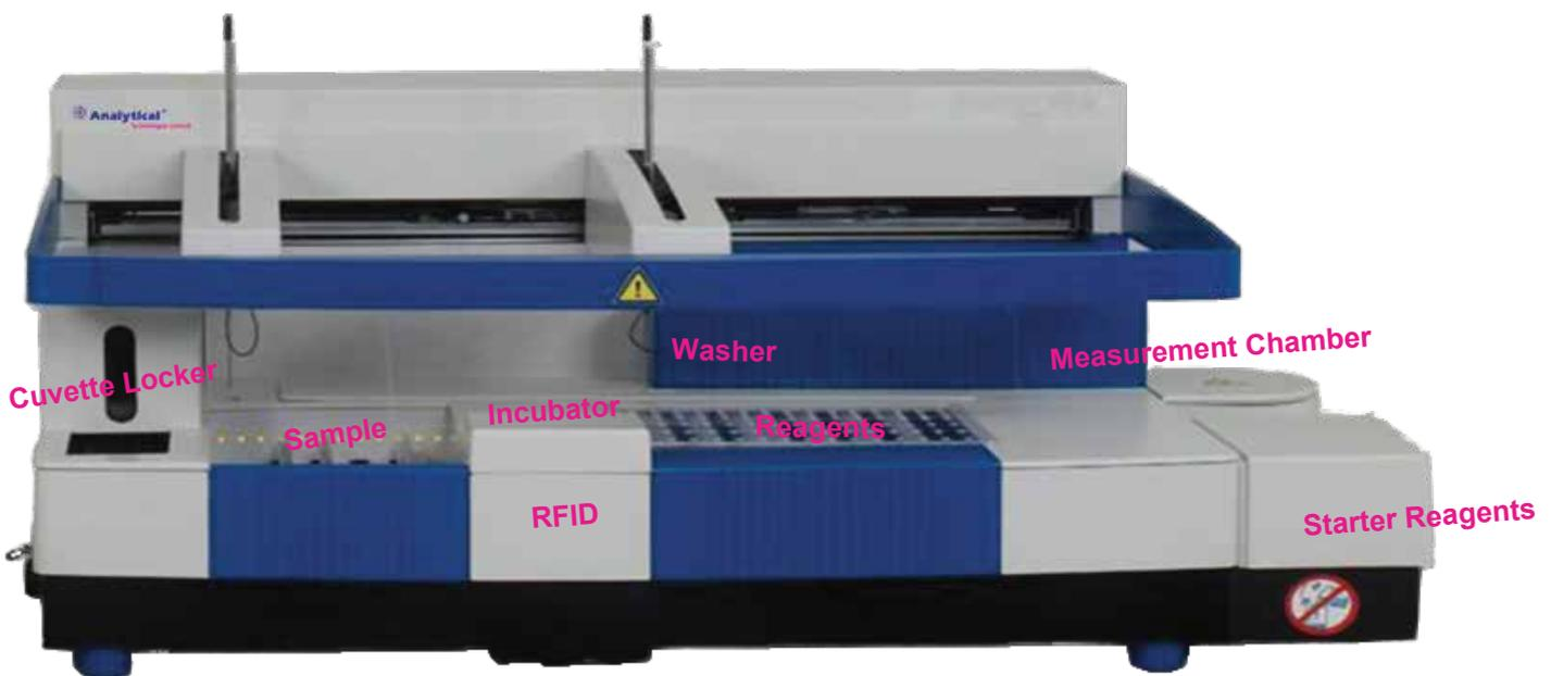
· Flash chemiluminescence ABEI label · Nano magnetic micro beads solid phase · Throughput : Maximum 120 tests / h · Sample and reagent continuous loading · On board capability : up to 144 samples · Random access or batch mode, STAT · 2-point calibration, stable for 4 weeks · 1 Titanium needle for sample and reagent · Refrigerated reagent area · On board capability : 15 analytes · Reagent recognition : RFID reader
